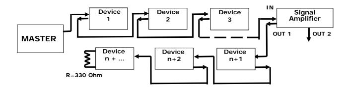
When the length of bus cable is more than 800 meters, install a signal amplifier. Put the resistance only in the last device in terminal block A-B.
