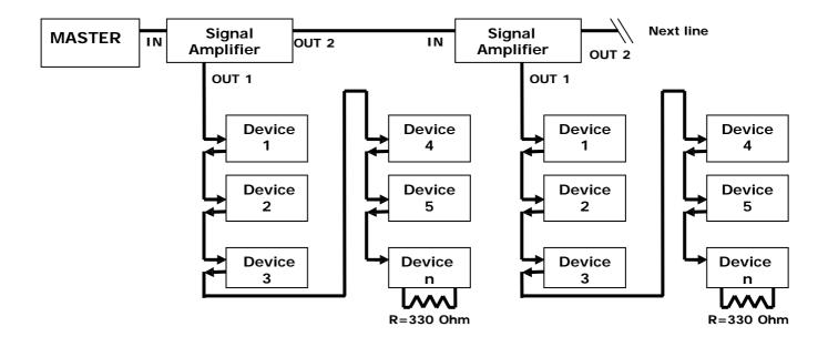
Put the resistance in the last device of each line, in terminal block A-B.
